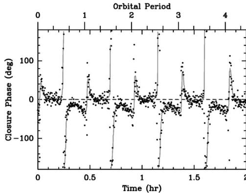
**Figure 3.** Simulated 230 GHz closure phases of a hot spot orbiting at the ISCO embedded in a quiescent RIAF disk ( $a = 0, i = 30^\circ$ ). The grey curve shows the model values for an array consisting of phased Mauna Kea (JCMT + CSO + 6 SMA dishes), phased CARMA (8 dishes), and the SMT. Black points represent simulated 10 second integrations at  $8 \text{ Gbit s}^{-1}$ .
