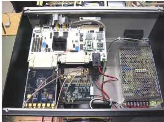
**Figure 1.** The Digital Backend (DBE) system developed to process two 480MHz wide IF bands, producing an aggregate VLBI data output rate of 3.84 Gigabit/sec.
